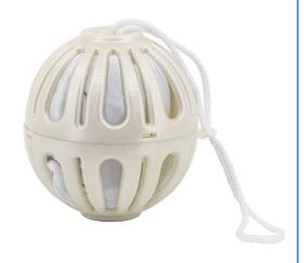
Multipure's Aquasplash works as chlorinated water flows through the KDF®-55 media inside the ball, creating an electrolytic reaction which causes the two chlorine ions to form a harmless chloride.
