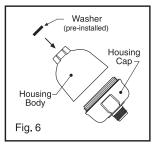
scale buildup in pipes is excessive, you may experience an early reduction in water flow. This may be an indication that you need to replace the cartridge more frequently than the recommended 6 to 7 months. For best results, the housing body should be replaced every 3 years or as needed.
