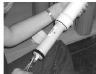
Step 3 Using a pair of pliers, grip and pull firmly on the membrane to remove from the housing and discard in your normal refuse.
