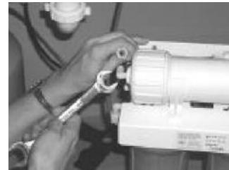
Step 2 Remove the cap from the white horizontal membrane housing. Use the hand tool shipped with the unit to loosen. Turn cap counter-clockwise to loosen.
